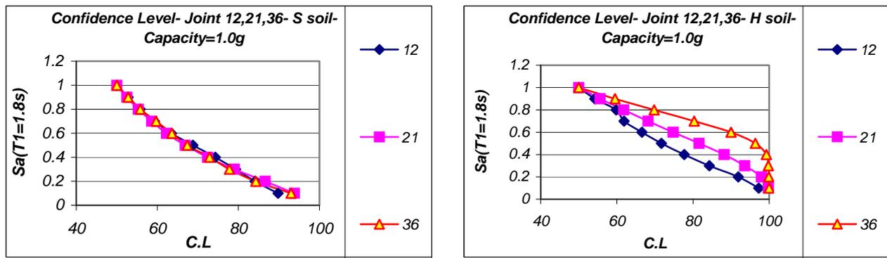
Figure 4. Results of confidence level by assuming capacity=1g, and comparison between different joints and soils
