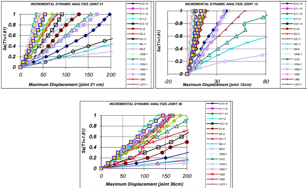
Figure 1. Incremental Dynamic Analysis for three different location of structure (joint 12,21,36)
