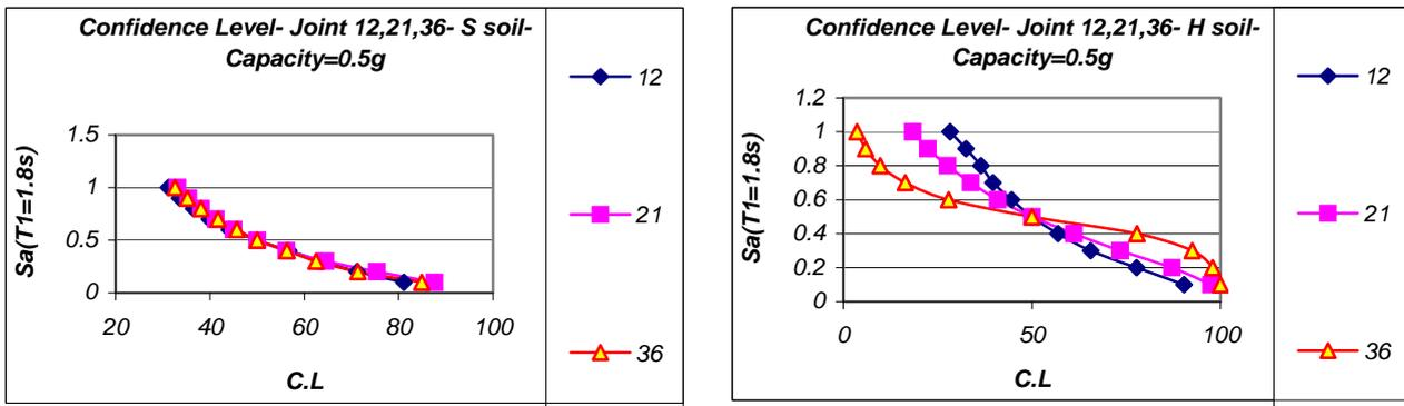
Figure 3. Results of confidence level by assuming capacity=0.5g, and comparison between different joints and soils
