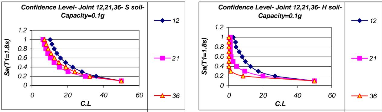
Figure 2. Results of confidence level by assuming capacity=0.1g, and comparison between different joints and soils
