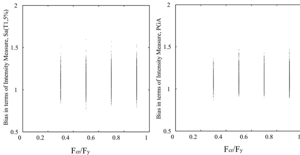
Figure -5. The bias in the SDOF seismic capacity points in terms of intensity measure versus  $F_{cr}/F_y$ . The alternatives for the IM are PGA and  $S_a(T_1, 5\%)$ .
