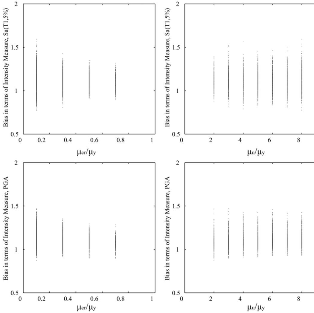
Figure -4. The bias in the SDOF seismic capacity points in terms of intensity measure versus  $\mu_{cr}/\mu_y$  and  $\mu_u/\mu_y$ . The alternatives for the IM are PGA and  $S_a(T_1, 5\%)$ .
