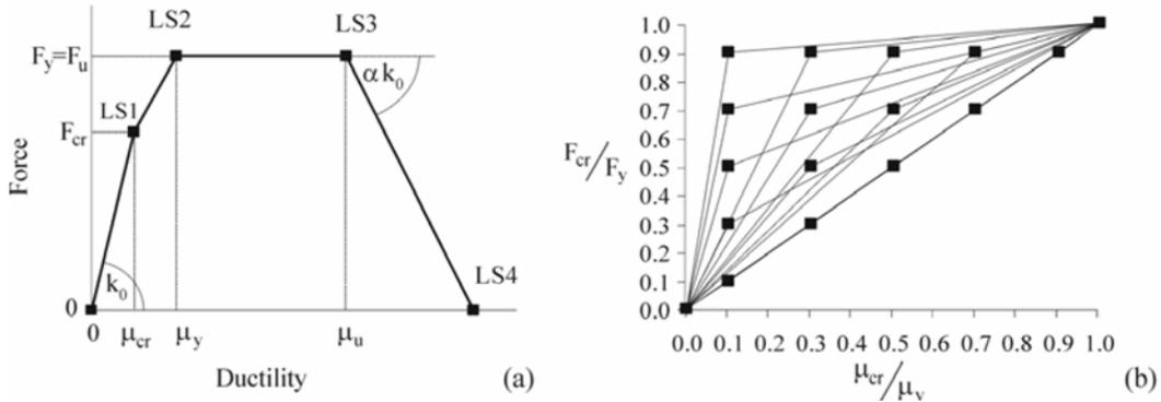
Figure -1. (a) Definition of the backbone curve with six controlling parameters (b) all different possible combination of the backbone curves for the ratios  $F_{cr}/F_y$  and  $\mu_{cr}/\mu_y$  between 0 and 1.
