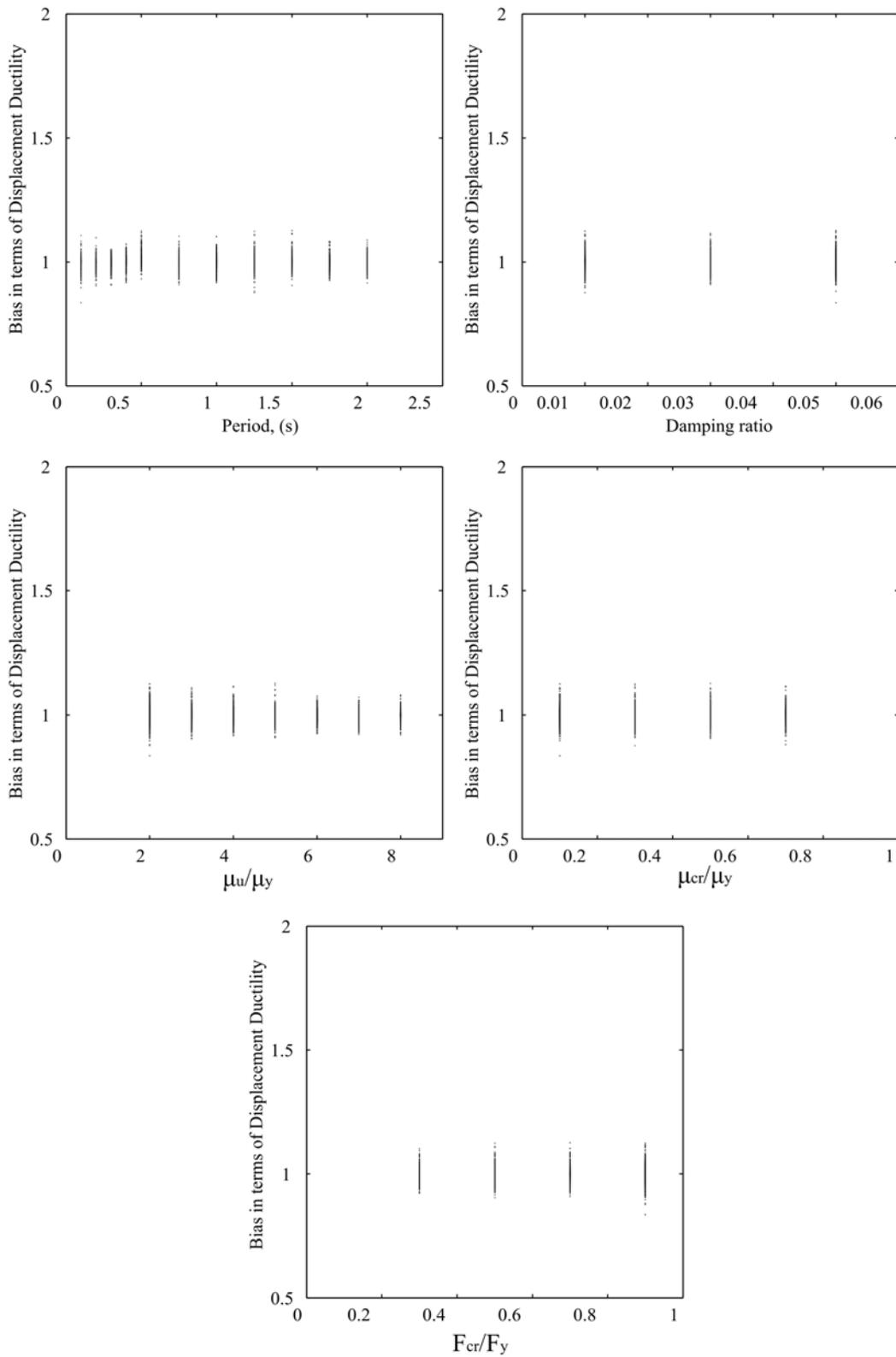
Figure -6. The bias in the SDOF seismic capacity points in terms of displacement ductility versus period, damping and backbone controlling parameters (see Figure 1).
