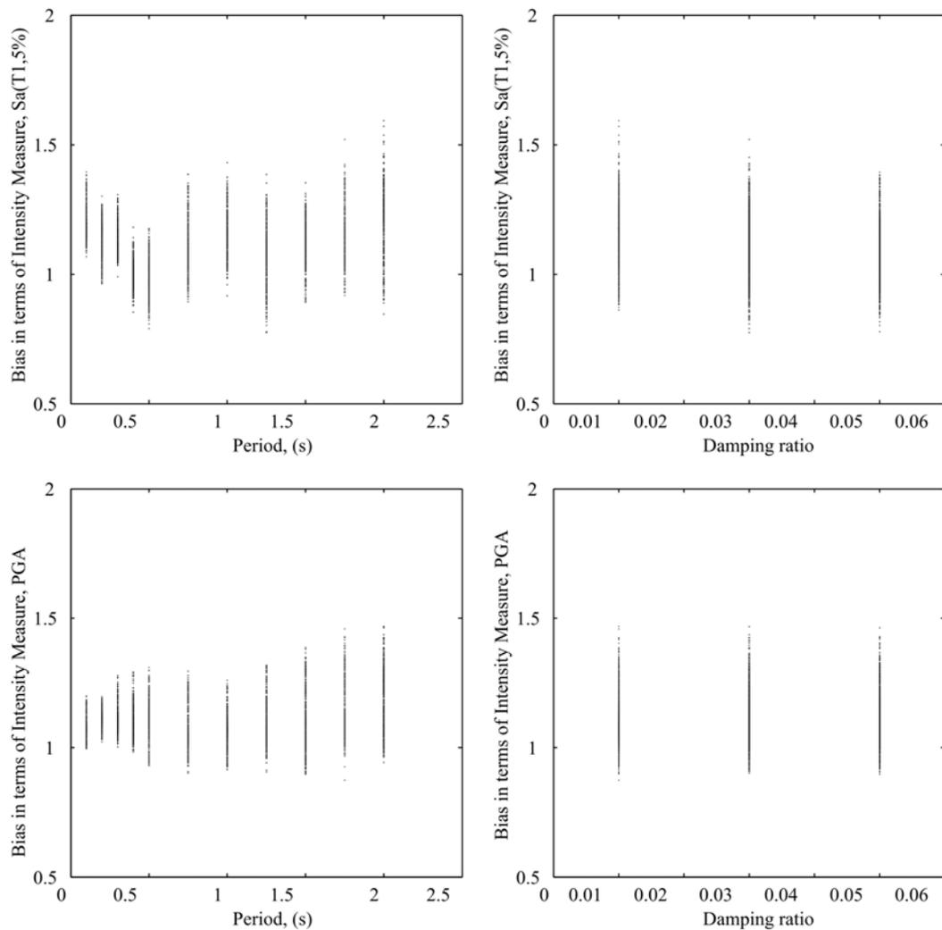
Figure -3. The bias in the SDOF seismic capacity points in terms of intensity measure versus period and damping ratio. The alternatives for the IM are PGA and  $S_a(T_1, 5\%)$ .
