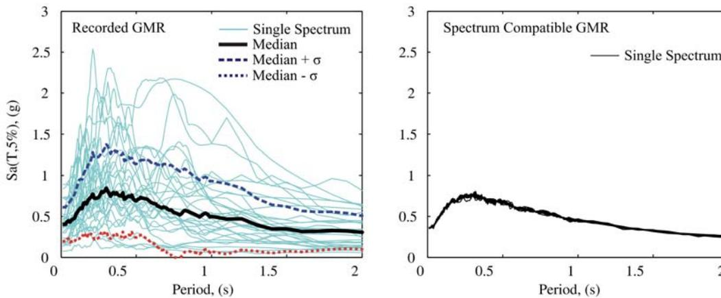
Figure -2. The 5% damped elastic response spectra for the 31 recorded (left) and spectrum compatible (right) ground motion records.
