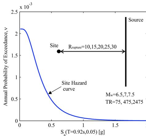
Figure 2. Different parameters used in sensitivity analysis and sample hazard curve for  $T=0.92$  s,  $M_w=7$  and  $TR=475$  years.
