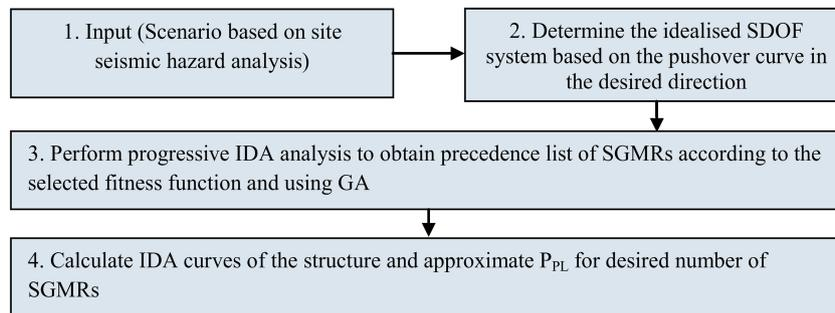
Figure 10. Steps involved in determination of  $P_{PL}$  using progressive IDA.
