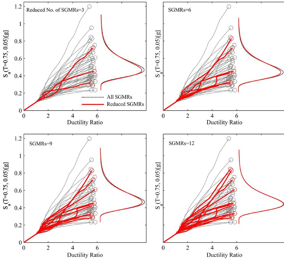
Figure 6. Effect of number of selected SGMRs on probability density function of collapse capacity using improved fitness function for an arbitrary system with  $T = 0.75$  s,  $\mu = 6$ ,  $\xi = 0.05$  and  $\alpha = 0.05$ .
