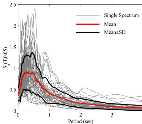
Figure 3. The elastic response spectra for the SGMRs, their mean and the mean  $\pm$  standard deviation.
