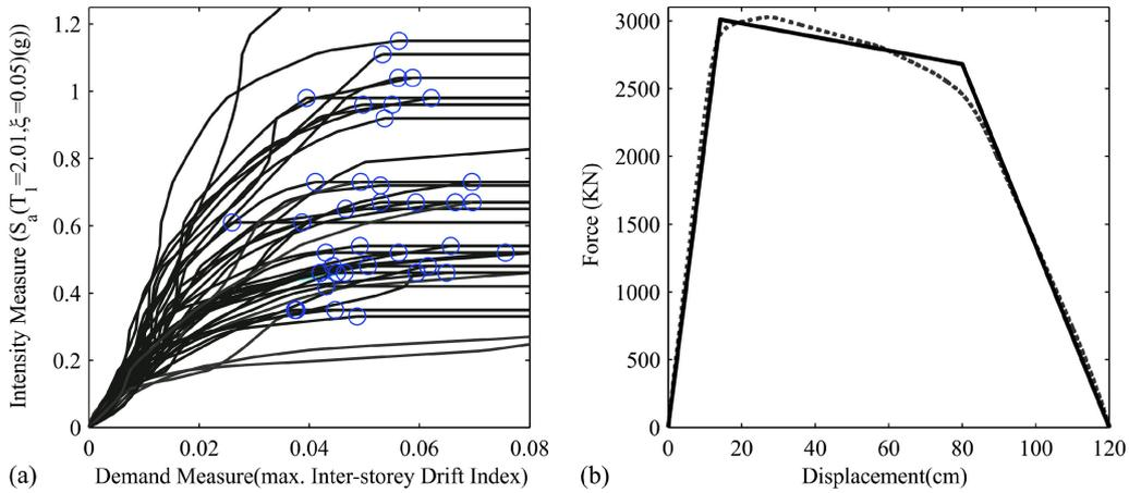
Figure 14. (a) IDA curves and (b) first-mode pushover curve and the equivalent idealized SDOF behaviour.
