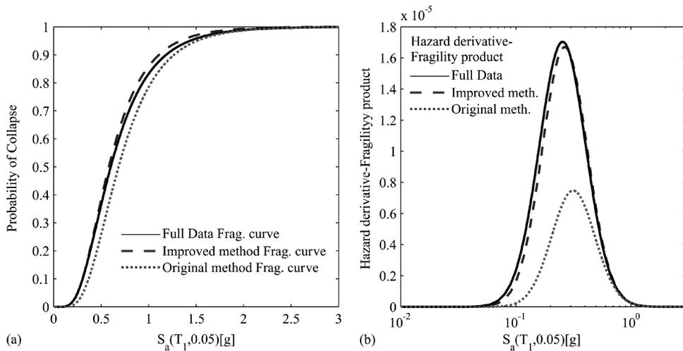
Figure 15. (a) Comparison of failure fragility curve using six SGMRs and different fitness functions and (b) comparison of hazard derivative-fragility product employing six SGMRs and different fitness functions.
