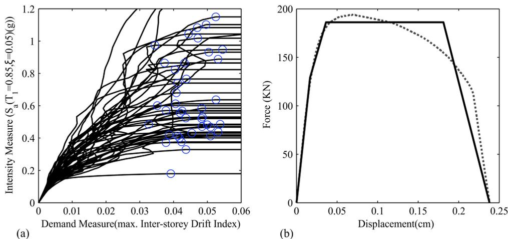
Figure 11. (a) IDA curves and (b) pushover curve in X direction and the equivalent idealized SDOF behaviour.
