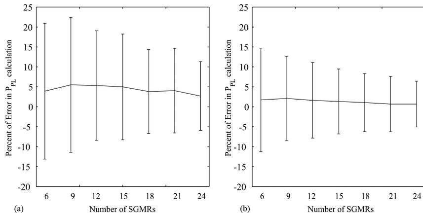
Figure 8. Comparison of error in  $P_{PL}$  calculation at 95% confidence level (mean  $\pm 1.96 \times$  (standard deviation)) for different number of SGMRs: (a) using original fitness function and (b) using improved fitness function.
