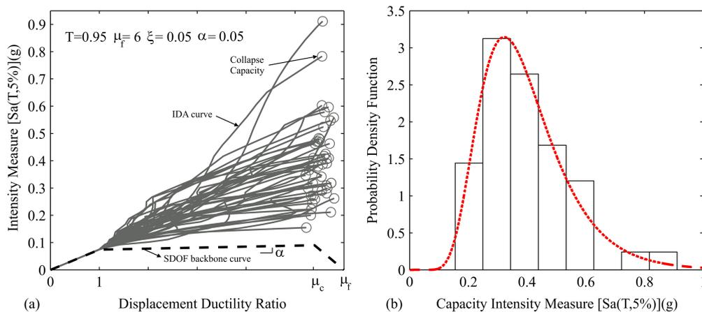
Figure 4. (a) IDA curves for a sample SDOF system with  $T=0.95$  s,  $\mu_f=6$ ,  $\xi=0.05$ ,  $\alpha=0.05$  and (b) the distribution of collapse capacity.
