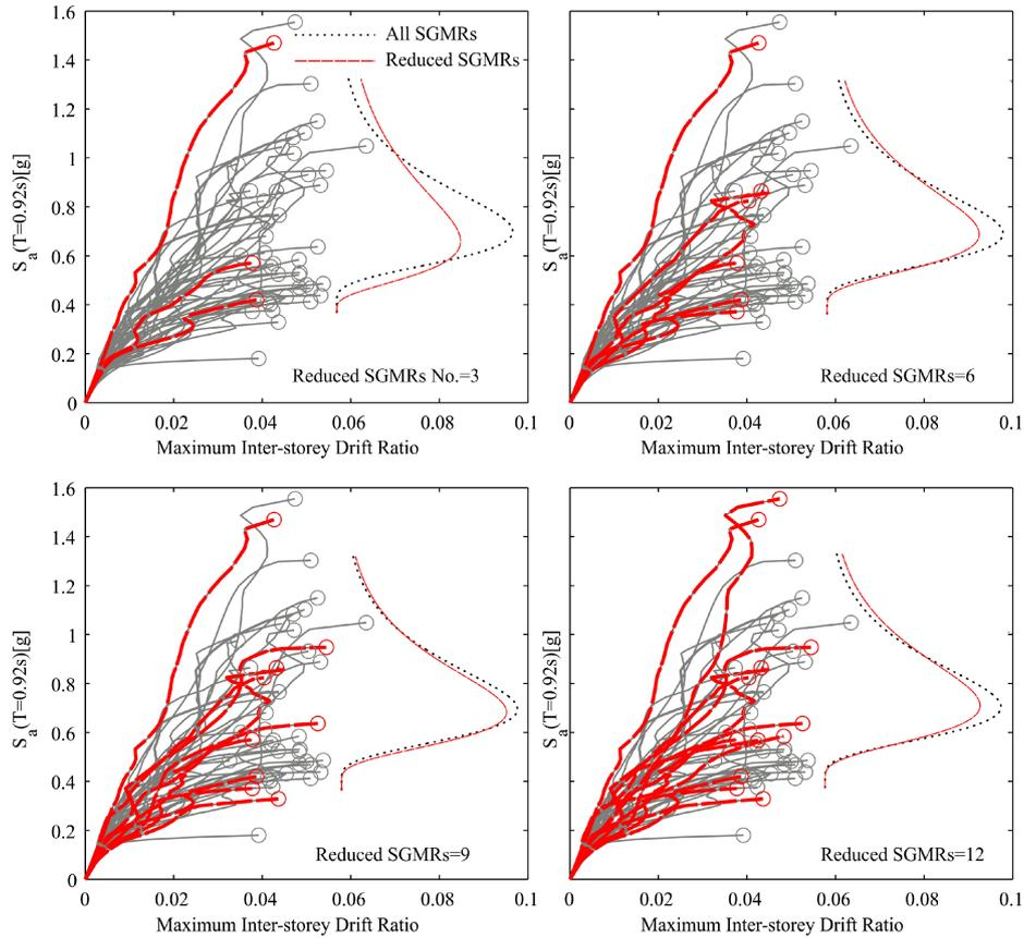
Figure 12. The effect of number of selected SGMRs on the probability density function of collapse capacity using the improved fitness function for the three-storey RC structure.
