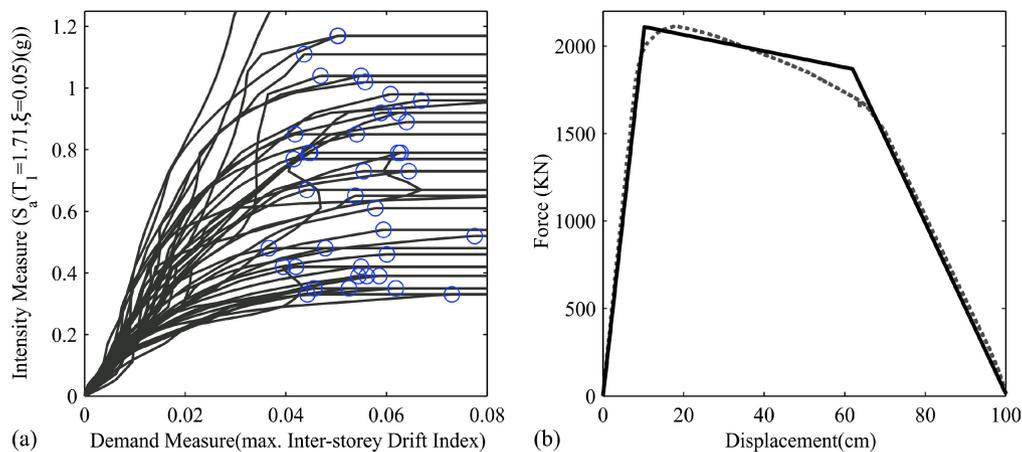
Figure 13. (a) IDA curves and (b) first-mode pushover curve and the equivalent idealized SDOF behaviour.
