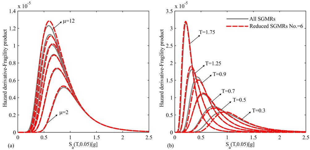
Figure 5. Hazard derivative-fragility product for  $M_w = 7$ ,  $R_{rupture} = 10$ ,  $TR = 475$  years: (a) SDOF system for different ductility values with  $T = 0.55$  s,  $\xi = 0.05$  and  $\alpha = 0.05$  and (b) SDOF system for different period values with  $\mu = 6$ ,  $\xi = 0.05$  and  $\alpha = 0.05$ .
