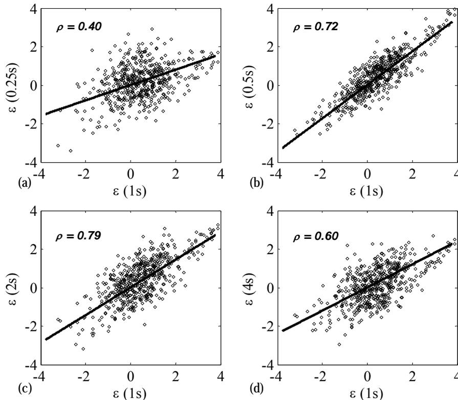
Fig 2. The Scatter plot of  $\epsilon$  values from a large set of ground motions.  $\epsilon(1.0s)$  versus (a)  $\epsilon(0.25s)$ , (b)  $\epsilon(0.5s)$ , (c)  $\epsilon(2.0s)$ , and (d)  $\epsilon(4.0s)$ .
