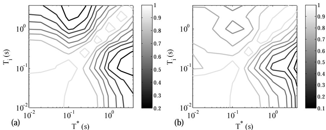
Fig9. Contours of correlation coefficients versus  $T^*$  and  $T_i$ ; based on (a) Conventional analysis (b) Robust correlation analysis.
