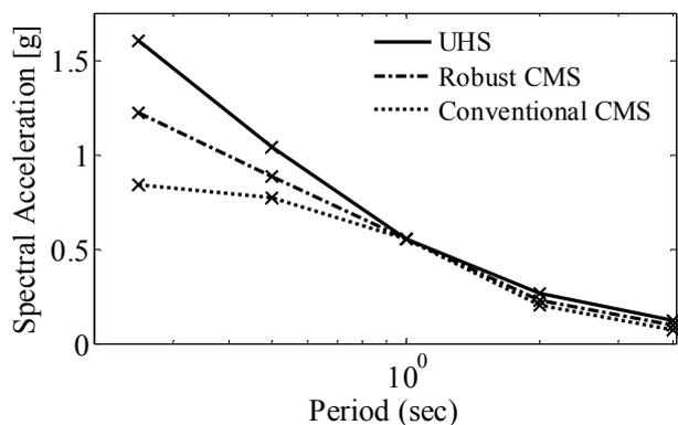
Fig 7. The comparison of the robust CMS with the conventional CMS.
