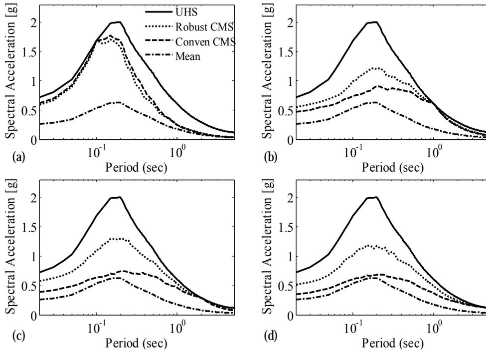
Fig 10. The robust CMS, conditioned on Sa values at the interest period.
