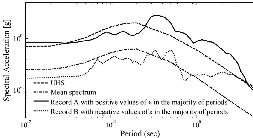
Fig 11. Comparison of two single records that have equal  $\varepsilon(4.0s)=+1.88$ , but different distribution of  $\varepsilon$  in the other periods.
