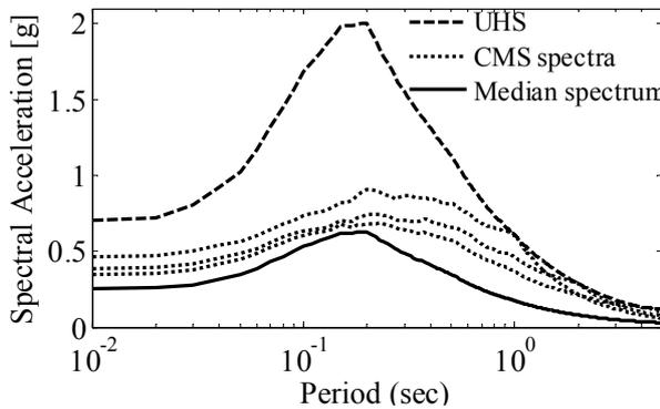
Fig 3. Conditional Mean Spectra, conditioned on Sa values at a few periods, having equal  $\varepsilon=1.88$ .
