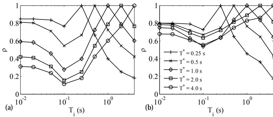
Fig8. Plot of correlation coefficients versus  $T^*$ , for several  $T_i$  values; based on (a) Conventional analysis (b) Robust correlation analysis.
